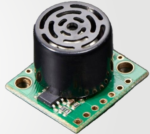
Figure 10: Ultrasonic Sensor Example LV-EZ4 Maxbotix Ultrasonic Rangefinder Source: Adapted from Image [6]
